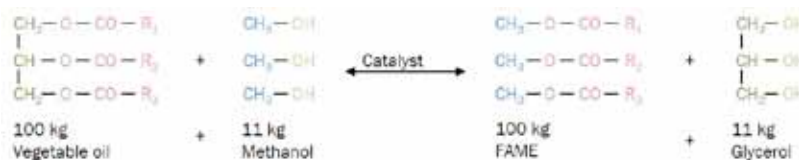
Fig. 3: Transesterification of vegetable oil to fatty acid methyl ester and an approximate mass balance of the transesterification.
