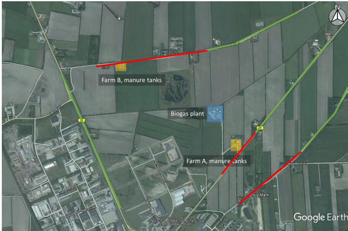
Figure 5: Geographical analysis of possible measurement locations as part of the planning of measurements. Green lines indicate possible, downwind measurement locations and red lines indicate locations, where interference from nearby, other sources of methane emission is considered a risk.
