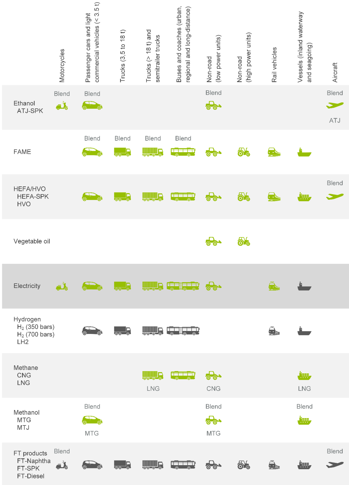
Figure 9-2 Vehicle-energy-matrix for Germany in 2030. Note: green – very probable option, dark gray – possible option, light gray – option for remaining stock of conventional drive systems; blend indicates blended fuels made of renewable and fossil energy carriers
