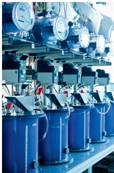
Fig. 61 Fully-mixed stirred-tank reactors in the DBFZ biogas lab
