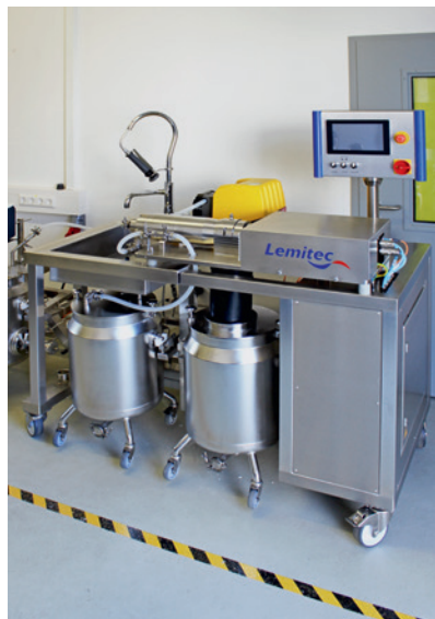
Fig. 64 New decanter test bed at the DBFZ's fuel technical centre
