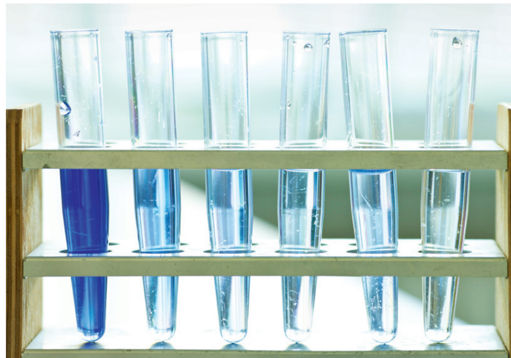
Fig. 45 Lowry protein assay at the DBFZ's biogas lab
