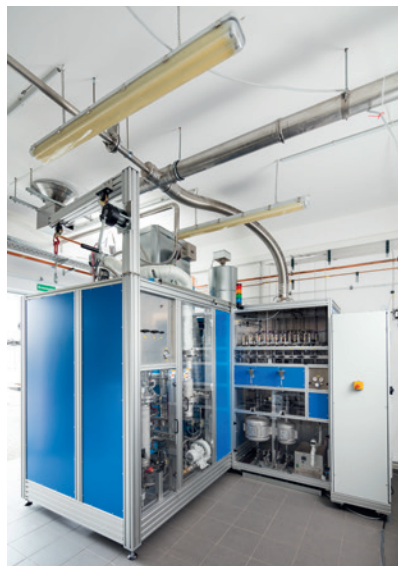
Fig. 63 Fixed-bed gasifier at the DBFZ's fuel technical centre
