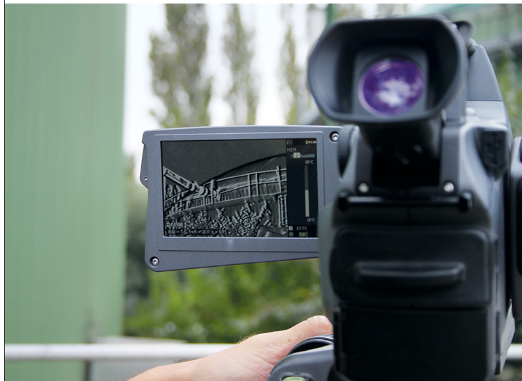
Fig. 9 Methane detection in a biogas plant
