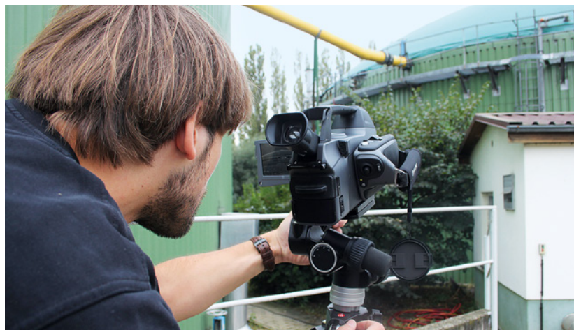
Fig. 5 Leak detection at a biogas plant
