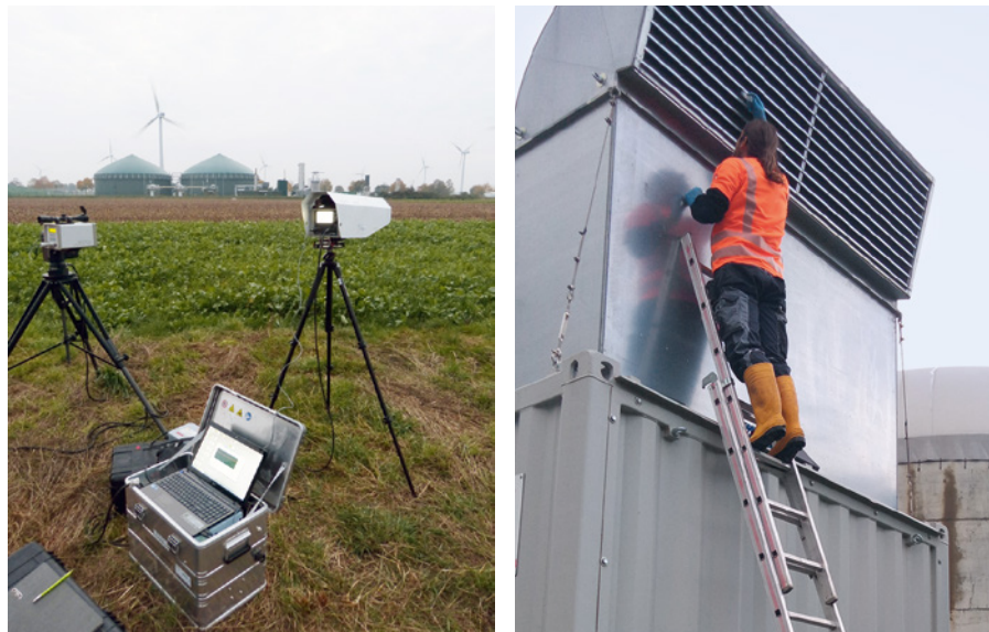
Fig. 7 Emission measurements at a biogas plant using the remote measurement method (l.) and on-site method (r.)
