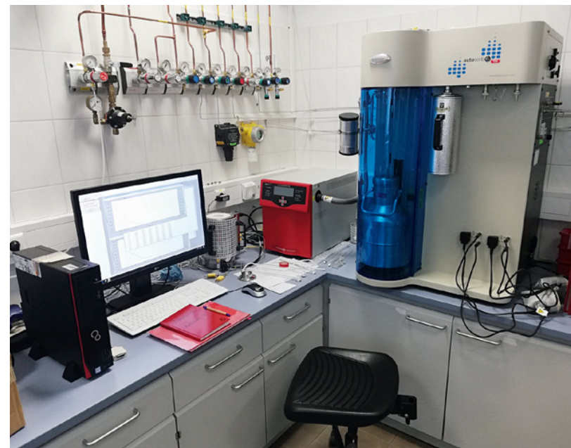
Fig. 14 Apparatus for the characterisation of solids (powders and monoliths) using methods of physical and chemical absorption.
