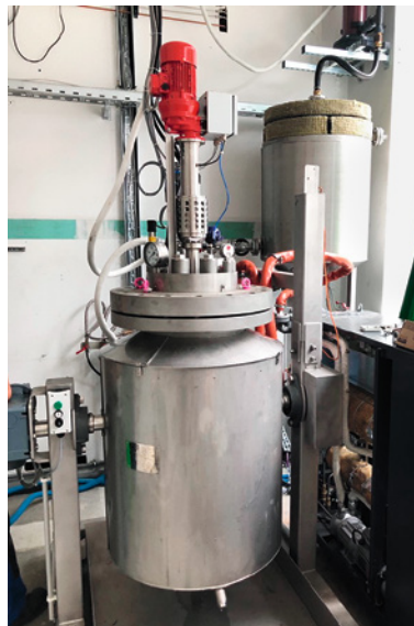
Fig. 14 100-L HTC reactor in the fuel technical centre of the DBFZ
