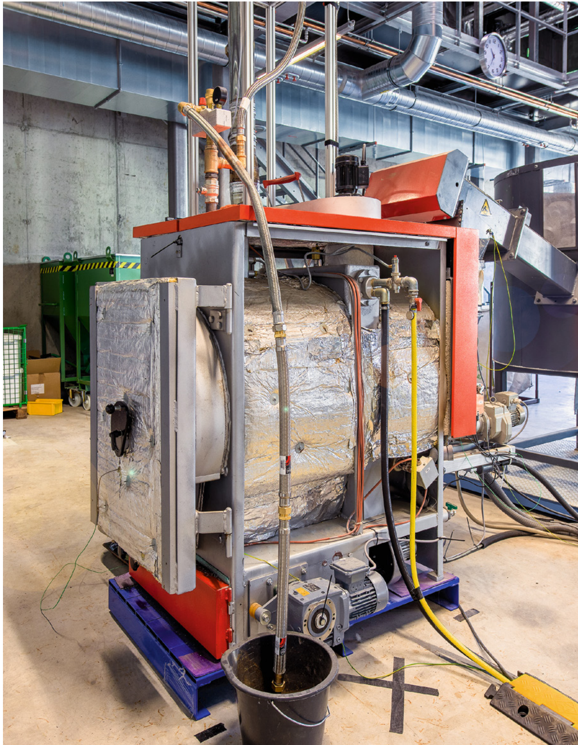
Fig. 19: Pilot plant for the production of biogenic silica from oat and spelt husks, model: Oekotherm 49 kW
