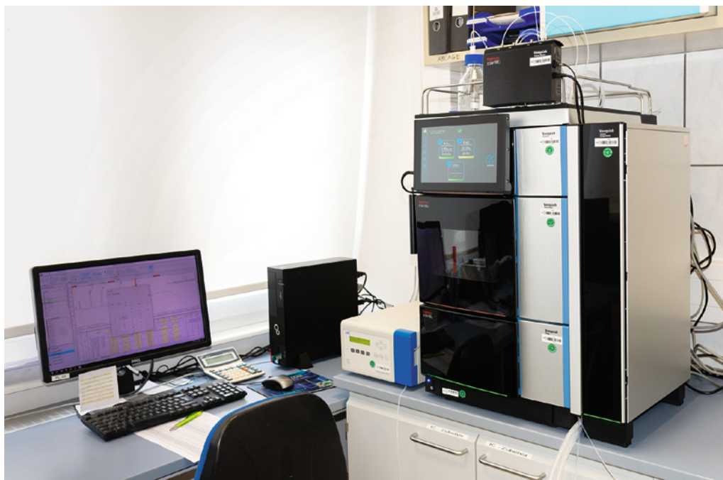
Fig. 41: New HPLC system in the DBFZ's analytical lab
