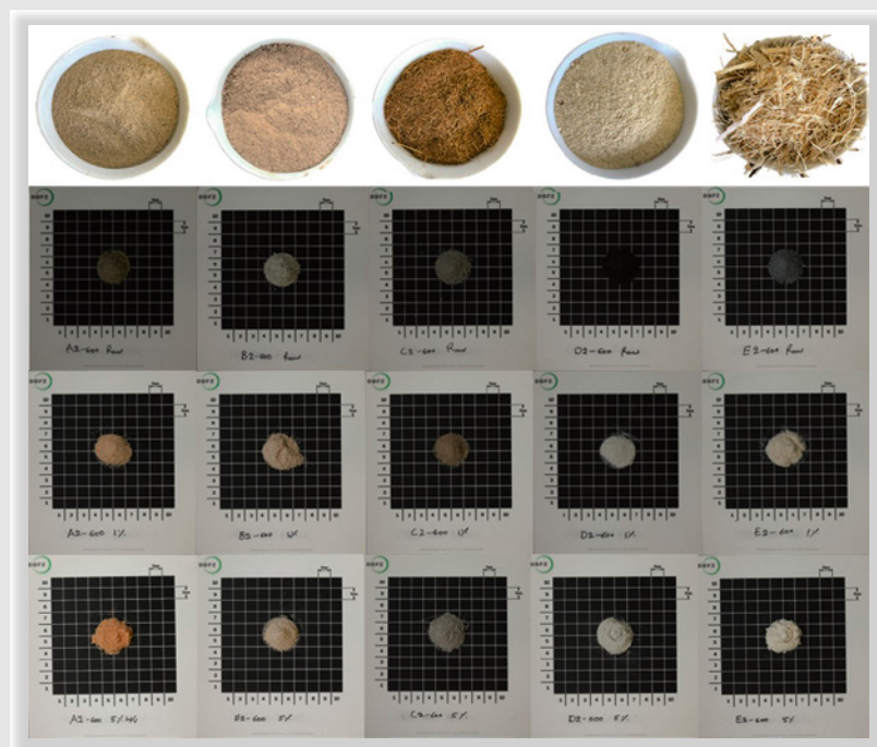
Fig. 31: Image overview of various thermochemically produced ashes from untreated and acid-leached African biomass residues at 600 °C. From left to right: biomass and ash from cassava peels, yam shells, coconut shells, maize cob spindle and maize straw. First row from top: untreated biomass fuels; second row: ash of untreated biomass fuels; third row: ash of biomass fuels with 1 ma.% acid wash; last row: ash of biomass fuels with 5 ma.% acid wash.
