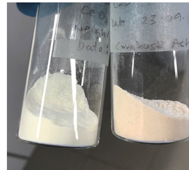
Fig. 32: Catalyst support material made from commercially available silica (left) and silica from corn husk ash (right)
