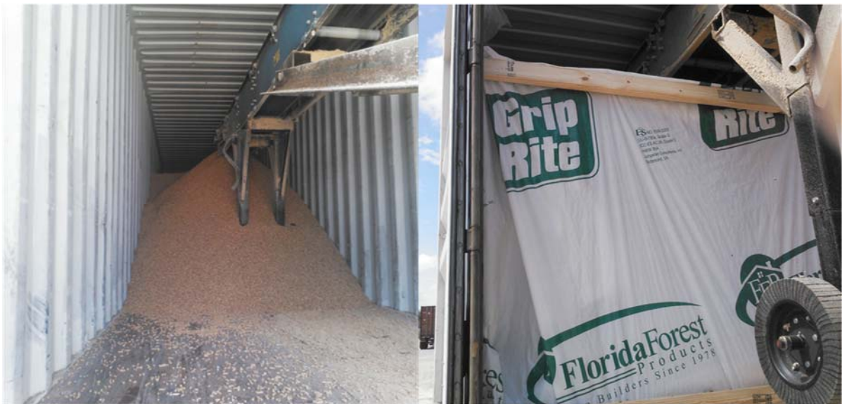
Figure 10 Loading (left) and sealing (right) of bulk transport in normed shipping container
