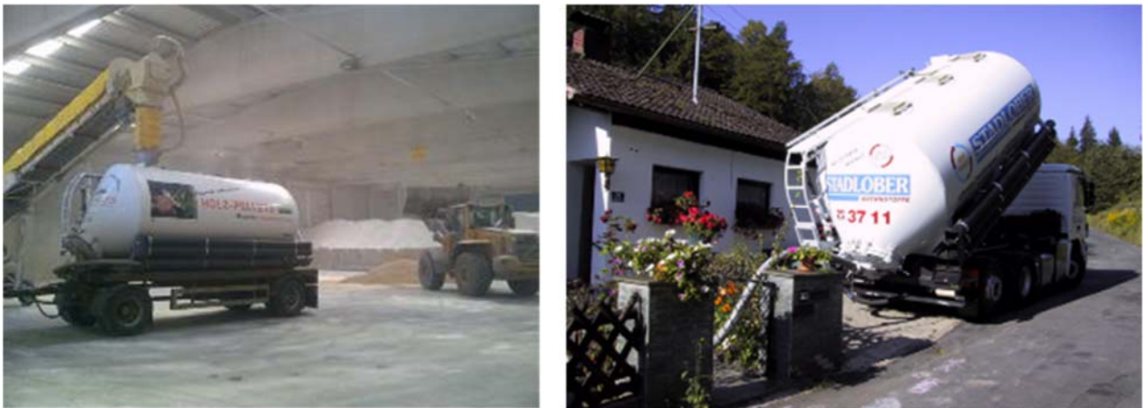
Figure 11 Pellet blower truck loading (left) and blowing into the cellar of a residential consumer (right)
